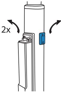
2. Push a cover plate in on both sides of the column.
