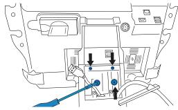
3. Connect the USB cable in the inner column to the USB port inside the stand head. Be certain that the USB cable is oriented correctly before pushing it in.
