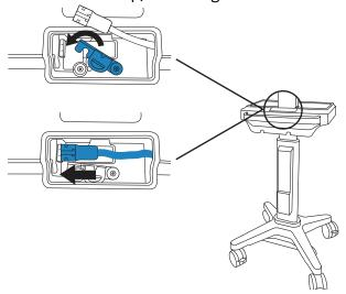
4. Place the lower part of the cover in first and then press down to lock it in place.
