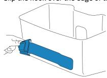
4. Slide the gel bottle holder down onto one of the mounting brackets on either side of the column.
