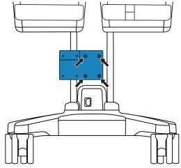
6. Slide the lip of the mounting box down onto the mounting bracket or stand, depending on which storage kit you have.
