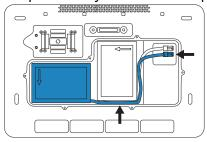
4. Attach the battery compartment cover with a Phillips screwdriver and the screws taped to the cover.
