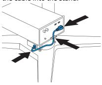
9. Connect the USB cable to the printer, and run the cable through the cable holder.
