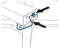
10. Plug the USB cable into the base of the stand and install the USB cover.
