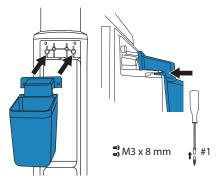
4. Snap the center gel holder cover onto the gel holder.
