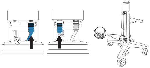
2. Push the cable connectors into place.
