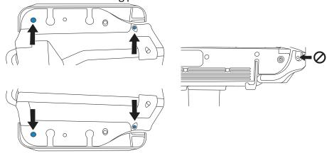
3. At the opening on top of the tray, turn the latch closed and then connect the video cable, with connector latch up, to the engine.
