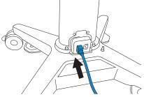
2. Run the AC power cord through the cord clip on the back of the storage tray. Wrap the cord if you need to wheel the system to an outlet.
