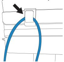
3. Connect the AC power cord to a hospital-grade AC mains outlet.
