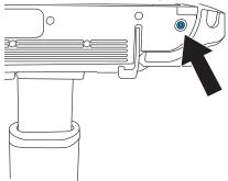
5. Make sure that the power status light on the base of the stand is on.
