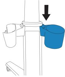
6. Use the #1 Phillips bit and two M3 x 8 mm screws to install the center gel holder at the top of the auxiliary stand battery.
