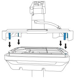
2. Use four M6  $\times$  12 mm screws and the 5 mm driver to secure the tray and monitor mount to the stand head. Insert screws from below the stand head into the monitor mount and tray. Do not use the rear mounting points.
