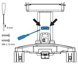
5. If you installed the four large storage bins, you must use the printer offset mounting bracket. Use the 4 mm bit driver and four M6 x 18 mm screws to install the printer mounting bracket to the stand.
