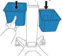
8. Connect the bins in pairs with a bin clip on each side.
