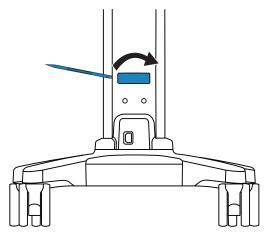
4. If you have the standard accessory kit, use the bit driver with the 5 mm bit and the M6 x 12 mm screws to attach the printer mounting bracket to the stand.
