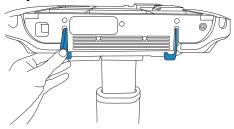
4. Secure the connection between the engine and the transducer connector by pushing the connector back into place, rotating the latch in the opposite direction, then pressing it up.
