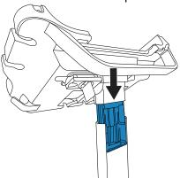
2. Use the bit driver with the 4 mm bit to tighten the four screws on the stand head.
