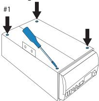
3. Remove the cover on the stand column with a pry tool.
