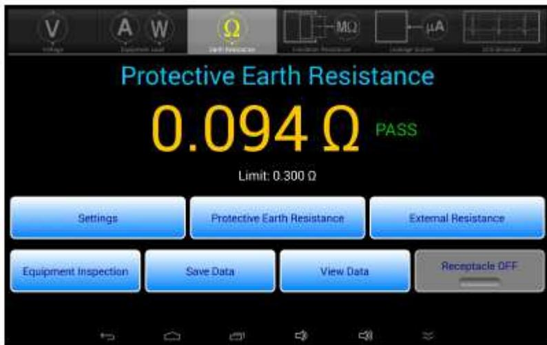
In the example of the CT Scan we consider today, according to the Manufacturer PM and IEC62353, the test needs to be performed on every protectively accessible conductive parts.
