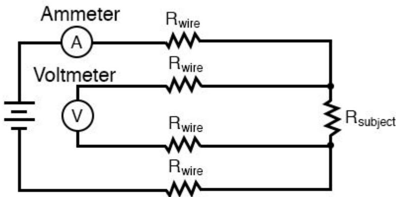
$$R_{\text{subject}} = \frac{\text{Voltmeter indication}}{\text{Ammeter indication}}$$
