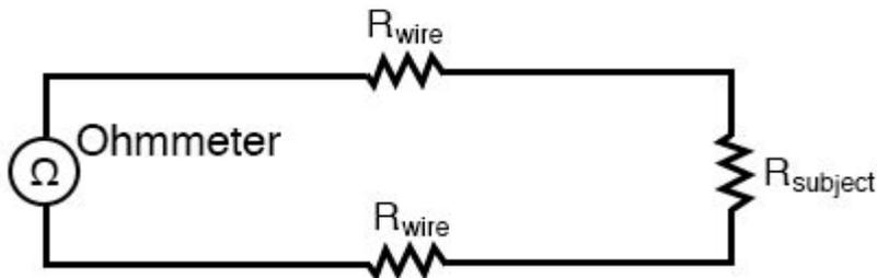
Ohmmeter indicates  $R_{\text{wire}} + R_{\text{subject}} + R_{\text{wire}}$
