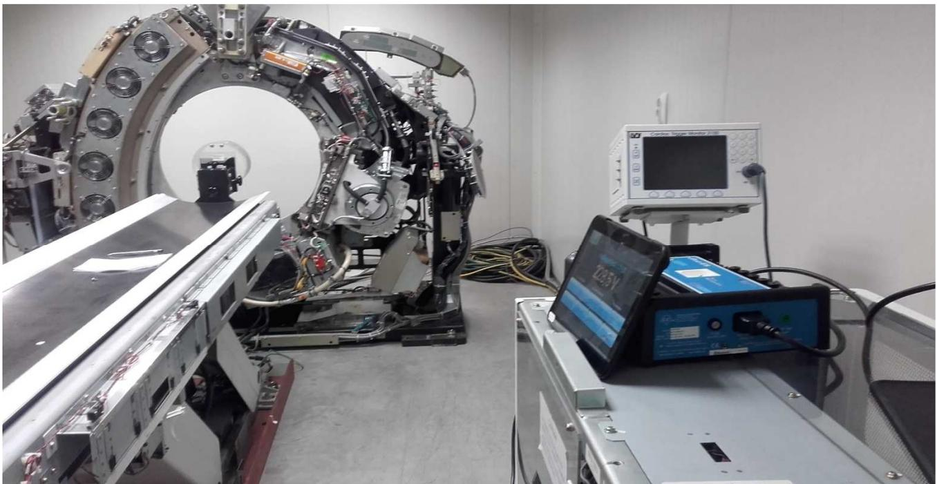
Due to the help of the kelvin technology used by Datrend Electrical Safety Analysers, the length of the cables used for this test do not have any impact of the measurement, even they are 10 meters long here on the example above.
